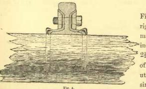
The scabbard-joint, Figs. 3 and 4, is more rigid, inasmuch as it makes a steel beam, 3½ inches deep, instead of 2½, has a greater mass of metal, better distributed; and is more simple, having fewer
